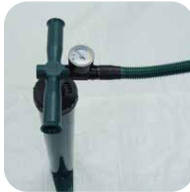
While holding the gauge, insert the hose and turn to lock. Check the hose end that goes in the valves, it should have hooks to lock it in the valve opening.
