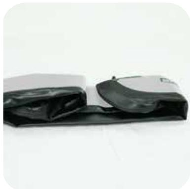
Fold the boat all the way to the end to push all the air out. Then unfold one fold. Fold bow back and place stern folds on top of bow. Use the seat straps to secure the folded canoe.
