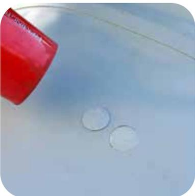
If you have access to electricity, heat the glue with a hair dryer then apply the patch. This method produces the best results. Mate the patch to the boat and smooth down until the patch adheres. Do not inflate, allow at least 24 hours to cure before inflating.
