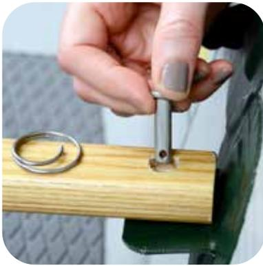
Align pin hole in line with sides of boat. Insert seat pins into frame hole and through grommet. **Note:** Careful alignment will make insertion of wire retainer ring possible.
