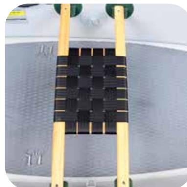
Adjust seat so holes in frame match seat grommets
