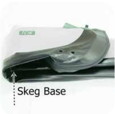
Make the first fold just after the skeg base. Continue folding toward the valves, pushing the air out as you go.
