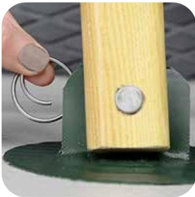
Find a comfortable position next to boat to install ring. Without looking under the seat, point inner end of wire ring towards hole in pin. Feel for hole in pin and insert wire into hole. Pushing the wire ring through the hole may be challenging at first but becomes easy with practice.
