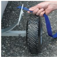
Place the rear of your boat on top of the EZ Cart and run the straps through the loops on the wheel frame.
