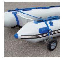
For most boat models you will only need to strap over the top of the boat. The straps make sure that the boat stays in place while you are pulling the boat. For larger models like our FoldCats & SailCat you can strap down each pontoon to the loop on the wheel frame.
