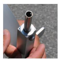
Begin by taking a washer and sliding it over the pins of the wheel frames.
