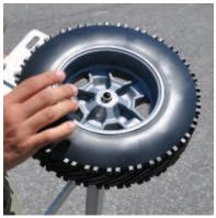
Next, slide the wheels over the washers and pins. Make sure the concaved side of the wheel is facing out, as shown.
