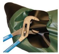
Place the material in the jaws of the channel lock pliers to protect the hull material. Once the body of is unscrewed from the base, pull the body from the opening and insert the replacement base. The opening is very tight, so you may have to pull on it hard.
