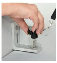
Secure the brackets to the motor mount block using one set of bolts. Orient the block so it hangs about 1/2" below the floorboard. Then use the remaining bolts to secure the mount to the floorboard.
