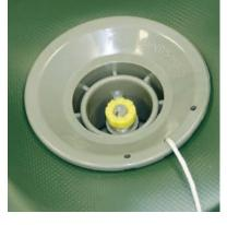
To deflate, remove the cap and press the valve stem down and clockwise into the open position. Release around 50-75% of the air from each chamber before fully deflating. Leave the valve open so excess air can be pushed out as you rollup the boat.
