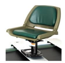
Now slide base of the swivel seat (or base of the pedestal if you are using it as shown) into the mounts. Make sure that the spring loaded lever mechanism locks into place.
