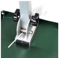
Before attaching the casting bar to your boat, make sure that the FoldCat's pontoons are partially deflated. Insert the upright bases over the underbars in the bow and tighten the set screws at the base using the hex key.
