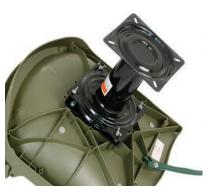
Bolt the upper end of the pedestal directly to the bottom of the swivel seat. Slide the other end of the pedestal into the release-a-seat mount and check to make sure that the spring loaded lever mechanism is locked.
