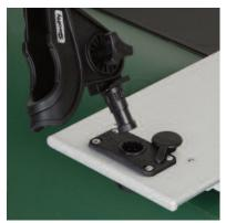
Next, install the rod holder into the base by pushing the post straight down into the mount. Line up the notch at the base of the rod holder with the key in the mount and insert it firmly into place. The rod holder can be roted in its base by lifting and turning.
