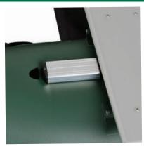
Align the ends of the underbars in line with the triangular markings on each pontoon.
