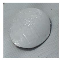
Apply adhesive to the dull side of the patch and around the area to be repaired. Coat the affected area lightly but completely with glue. If available, heat the glued surfaces with a hair dryer.
