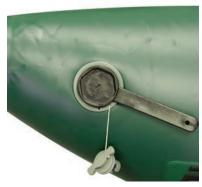
Inflate the chamber to full pressure if possible and loosen with the valve wrench by turning it counterclockwise. Deflate the chamber and unscrew the valve body from the base.
