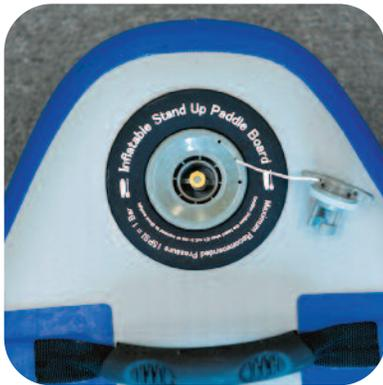
Remove the caps, press and turn the valve stems counter-clockwise so that the stem is in the UP position. When the stems are in the up position the valve will retain air. The LongBoard has a working pressure between 12 and 15 PSI. Do not exceed 15 PSI.
