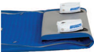
Make the next fold which will bring up the skegs. Place the skeg protectors over the skegs to protect them from being folded over.
