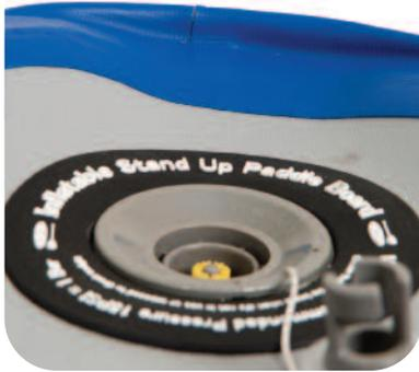
To deflate, push down on the center valve stem and quarter turn it to the right. The stem will stay in the down position, allowing the air to escape. Be sure that your eyes and your face are not directly over the valve.
