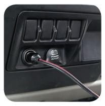
First, make sure the pump is switched *OFF* before inserting the power adapter into car's power outlet.
