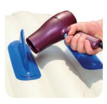
Using a hair dryer, warm the skeg until the curve becomes soft & pliable. This should only take about 2-3 minutes on a normal setting. Once the skeg(s) is soft, you can straighten it with your hands.
