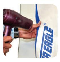
Use a hair dryer on the high setting to activate the adhesive and then press firmly on the patch until it cools.
