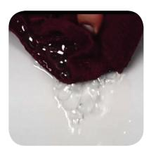
Soapy Water Test Inflate the boat to full pressure. Mix a couple of
