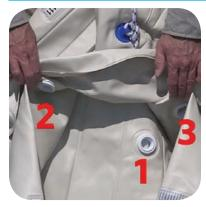
Locate the 3 main valves at the stern (back). Labeled in the photo is the floor chamber (#1), and the two side chambers (#2 and 3). Use the plastic inflation monitor to ensure proper inflation.
