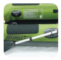
For quick access, with the oar in the oarlock, secure the shaft with the hook & loop strap.
