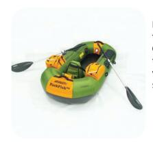
Repeat assembly for the other side. Orient the curve of the blades to cup the water on the power stroke.
